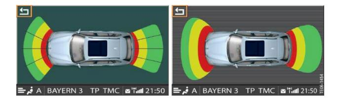
The park distance control is shown in the central information display when visual distance signalling and park distance control have been activated.
